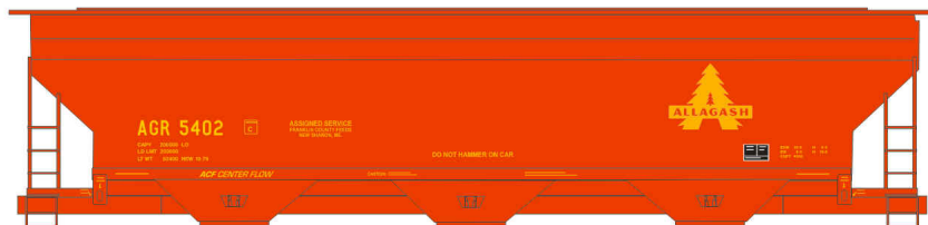
Typical Layout for Allagash ACF Center Flow 4650 CUFT Covered Hoppers. Carbody is all Red. Car Series 5400-5449 used in Grain & Corn Service.
