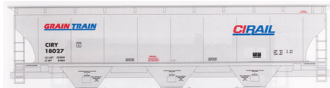
Owner: Eric Rissman Railroad: Central Illinois Rail Time Period: Modern Day Equipment Type: Trinity 5161 CUFT Covered Hopper (Atheam, LBF) Carbody is light gray.
